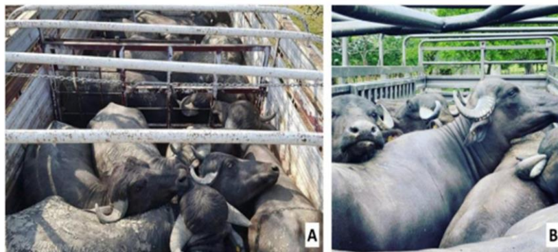
Figure 3 Physical adaptations of vehicles used to transport water buffaloes. A. A truck with the recommended load density reduces the risk of falls and injuries due to the space provided per animal. It is equipped with physical divisions to transport animals of different ages, sizes, or origins. B. Vehicles with a roof design provide ventilation but do not open any means of escape.
