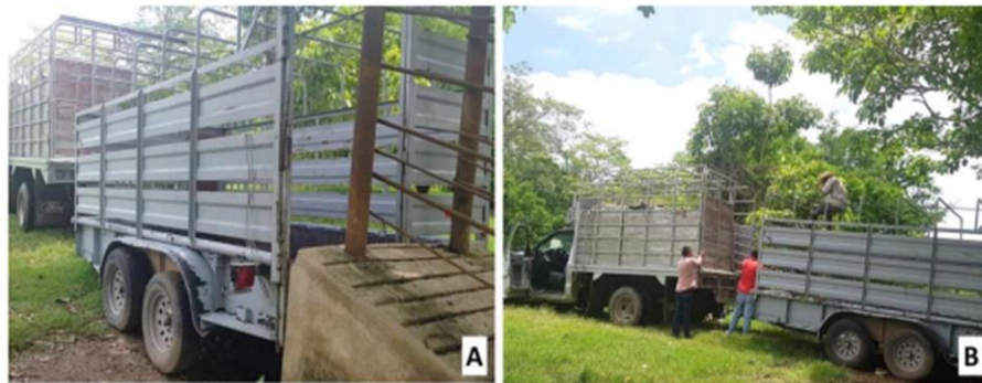
Figure 7 Loading and unloading ramps used in Mexico for buffalo transport. A. Trailer and uneven ramp. Though it has slots and an adequate slope, this ramp is not aligned correctly with the trailer, a factor that may cause injuries to the buffaloes' hind limbs. B. Type of trailers used to transport buffaloes in Mexico.
